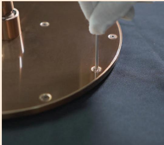
Twist the bolt open on the top side of the head shower with hex key.
